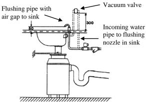
The figure above shows the positioning of a vacuum valve above a sink assembly. In your case the assembly used may be of another type (not a sink). The positioning of the vacuum valve will however remain the same
