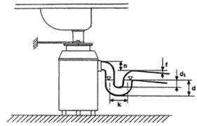
The figure above shows slope of the drain pipe. For specific installations the disposer may not be of the type shown above. The slope of the drain pipe will however remain the same.
