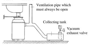
In installations where the disperator is evacuated by means of a vacuum, **no water trap** shall be connected to the outlet of the disperator. Instead, the disperator is connected directly to the collection tank of the vacuum system. It is important that the drain pipe between the disperator and the collection tank has a **ventilation pipe that is always open** as shown in the figure above. A ventilation pipe must be fitted even if the collecting tank has automatic airing.
