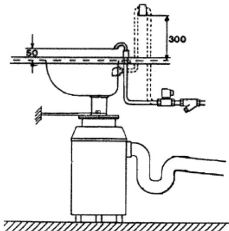
This figure shows the installation of a vacuum valve above a sink assembly. In your case the assembly used may be of another type (not a sink). The positioning of the vacuum valve is however the same.
