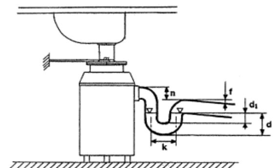
The figure above shows slope of the drain pipe. For specific installations the disperator may not be of the type shown above. The slope of the drain pipe will however remain the same.
