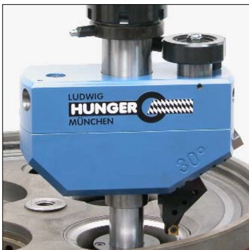
Valve seat refacing
