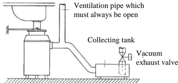
In installations where the disperator is evacuated by means of a vacuum, **no water trap** shall be connected to the outlet of the disperator. Instead, the disperator is connected directly to the collection tank of the vacuum system. It is **important** that the drain pipe between the disperator and the collection tank has a **ventilation pipe that is always open** as shown in the figure above. A ventilation pipe must be fitted even if the collecting tank has automatic airing.
