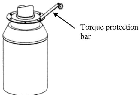
When starting or stopping quickly (e.g. if cutlery mistakenly jams the grinding unit) the torque of the motor will cause the disperator to turn. This may move the drain pipe / water trap from its position causing water leakage. A torque protection bar can be ordered, as an option, from Disperator if not available on installation site. When ordering please specify the distance between wall / bulkhead and suitable fixing screw on the upper disperator flange as per figure above.
