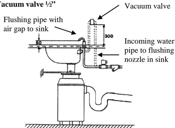
The figure above shows the positioning of a vacuum valve above a sink assembly. In your case the assembly used may be of another type (not a sink). The positioning of the vacuum valve will however remain the same
