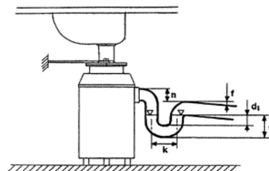
The figure above shows slope of the drain pipe. For specific installations the disperator may not be of the type shown above. The slope of the drain pipe will however remain the same.
