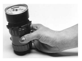
7. Clean the reaction vessel with the optional Zematra Water Free Cleaning Spray.
