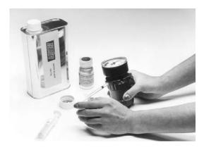
Place the reaction vessel on the magnetic stirrer and switch the stirrer on. If a heater / stirrer is used, turn off the heater. Read the manometer after 10-12 minutes.
